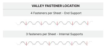
NOTE: Side lap fasteners are optional when using 5 fasteners per sheet, but are a requirement when only using 3 fasteners per sheet for valleys.
